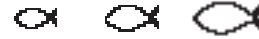
83 kHz, Wide Beam and 455 kHz Side Beam Hollow Fish Symbols (DualBeam PLUS™ and QuadraBeam™ Only)
